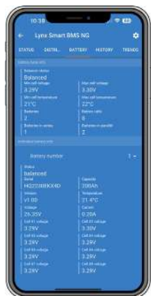
Complete overview of all battery data via VictronConnect (or a GX device and VRM)
